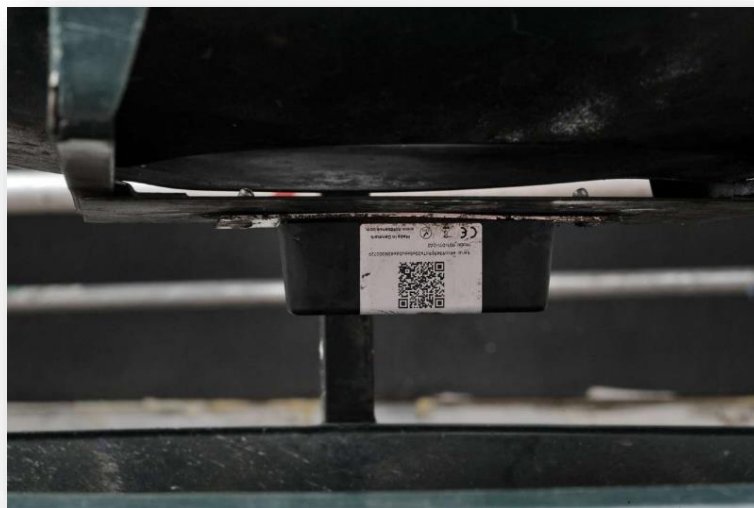
Photo 22: Close-up of Sensor Installed in San Francisco Public Space Waste Containers
